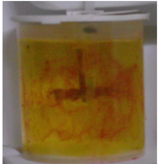
Fig. (17): Effect of the Speed Reduction on the Colors Zones of the Acid-Base Visualization Method Test, (a) 100rpm and 0.04m Impeller Diameter, (b) 50rpm and 0.04m Impeller Diameter.
